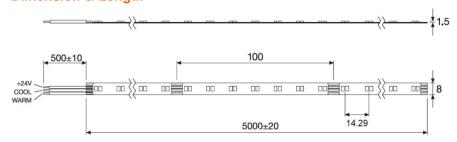
Lowest Bending Radius = 20mm Number LED/m = 140 Pre-soldered wires on one side
